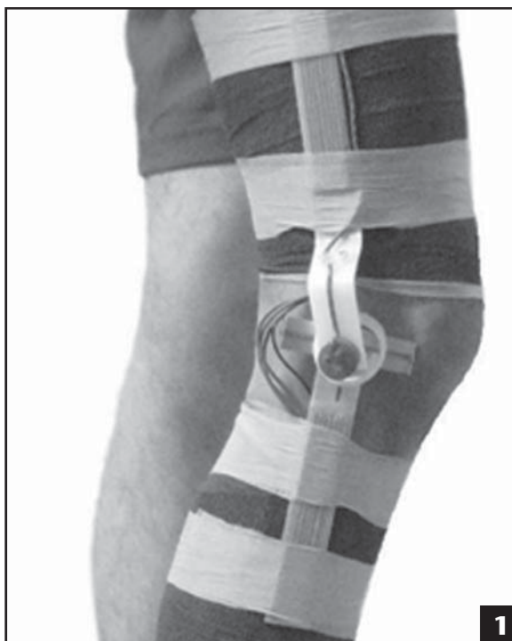
Figure 1. Custom-built electrogoniometer, attached to the lateral side of the knee joint of the dominant leg.
